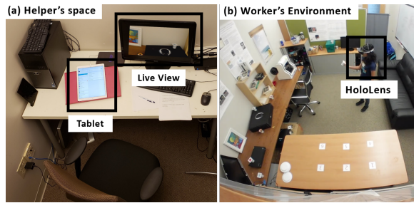
Figure 2: Helper's space and worker's environment. (a) The helper has a live first-person view of the worker throughout the experiment, and a specific aid (map or list) on a tablet. (b) The worker wears a HoloLens throughout the experiment, regardless of whether guidance is present or not.
